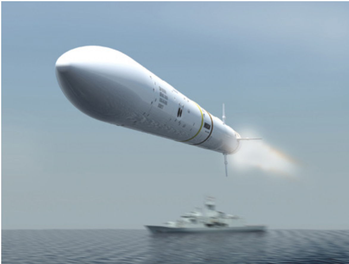
The Sea Ceptor is a sea-based supersonic missile defence system, fitted to HMNZS Te Kaha and HMNZS Te Mana | Credit: MBDA missile systems
